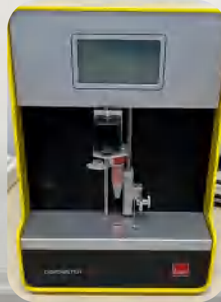
OSMOMETER Osmolarity determination
