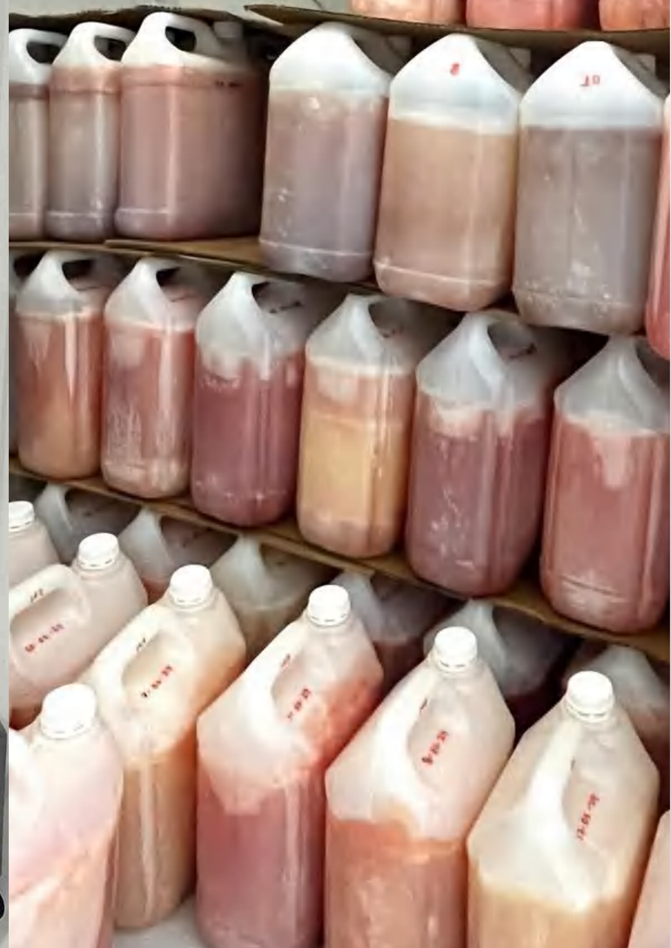
Raw serum is placed in 4.25 kg containers and stored in the raw material chamber at -18^{\circ}\text{C} ❄️
